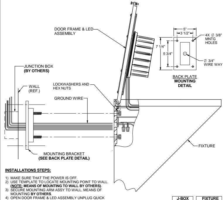
4) OPEN DOOR FRAME & LED ASSEMBLY UNPLUG QUICK DISCONNECTS REMOVE FROM HOUSING AND SET ASIDE.
